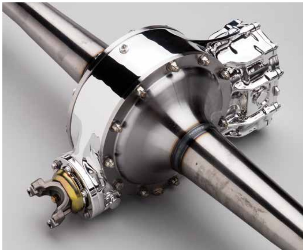
Rated for 800+ horsepower, the Champ quickchange is the largest Winters street rear, with a 10-inch, 4.12 ring and pinion and a gear drive track differential. This steel tube and bell version has a polished center, but they're available in a cast finish as well. They're equipped with axle housing flanges for 31-spline big bearing and big bearing "Torino" axles, and can be run with OEM-style drum or disc brakes.
