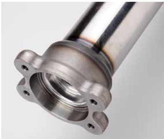
Rated for 800+ horsepower, the Champ quickchange is the largest Winters street rear, with a 10-inch, 4.12 ring and pinion and a gear drive track differential. This steel tube and bell version has a polished center, but they're available in a cast finish as well. They're equipped with axle housing flanges for 31-spline big bearing and big bearing "Torino" axles, and can be run with OEM-style drum or disc brakes.
