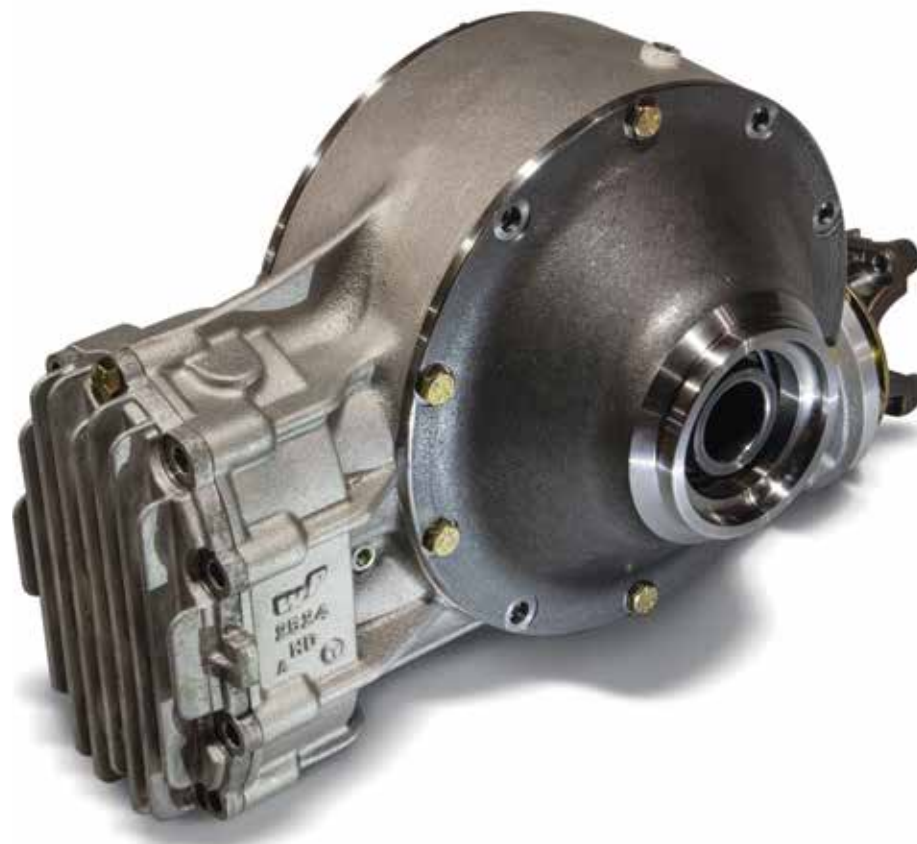
The smaller V8 quickchange is shown with forged bells prior to the steel tubes being welded in place. These are rated for 550hp and use an 8-3/8-inch, 3.78 ring and pinion and a Wedglock differential. Shown here is the straight-fin gear cover with a cast finish. Particularly when fully polished and fitted with the gusseted rear cover, the latest Winters V8 quickchange really takes on a vintage look.
