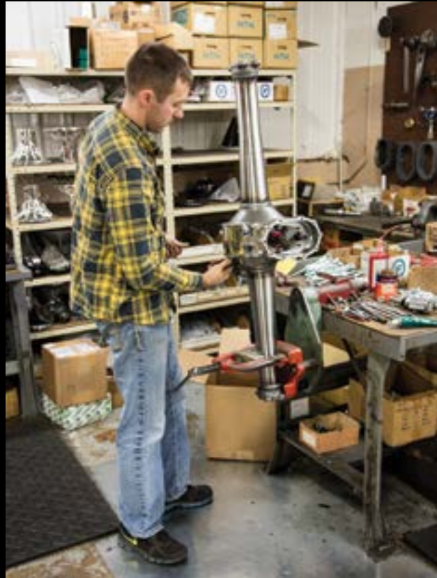
We've never seen so many quickchanges in one place as we did while touring Winters' facility. With the exception of the housing castings, which are done in Ohio, and a few select components the rears are made entirely in-house.
