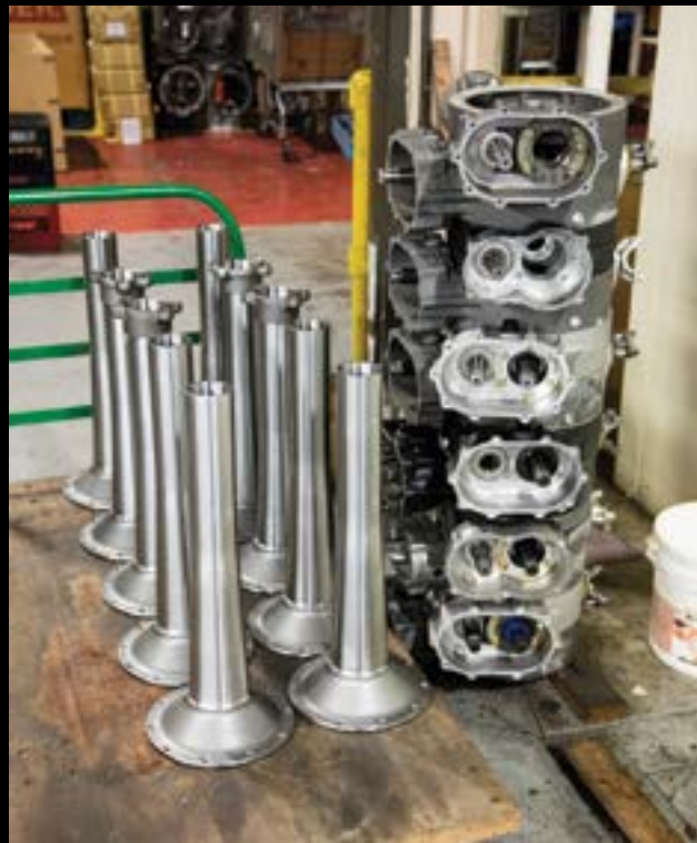
We've never seen so many quickchanges in one place as we did while touring Winters' facility. With the exception of the housing castings, which are done in Ohio, and a few select components the rears are made entirely in-house.
