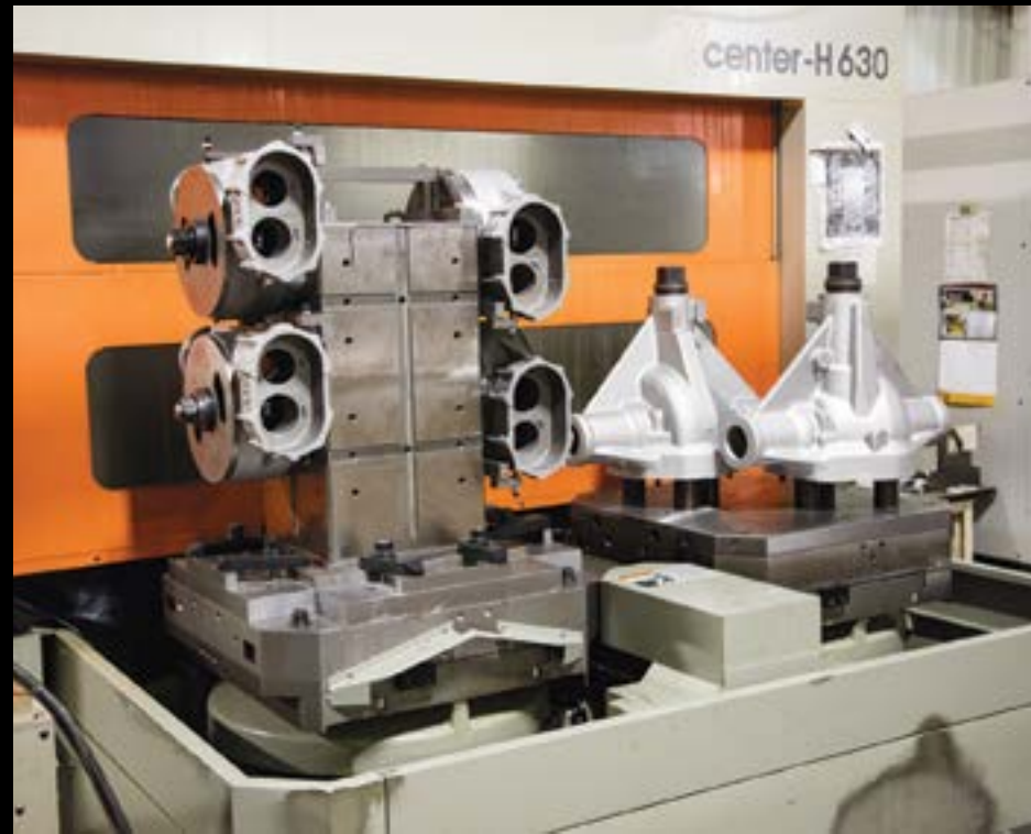
Raw castings are loaded into a CNC machining center for operations ranging from boring and drilling to facing and decking mounting surfaces. On the left are V8 quickchange centers and at right are aluminum Dana 60 housings they also manufacture. Winters has always invested in new technology and equipment that allows them to produce their rears more efficiently, but they also rely on skilled craftsmen to run that equipment and handle other manual processes.
