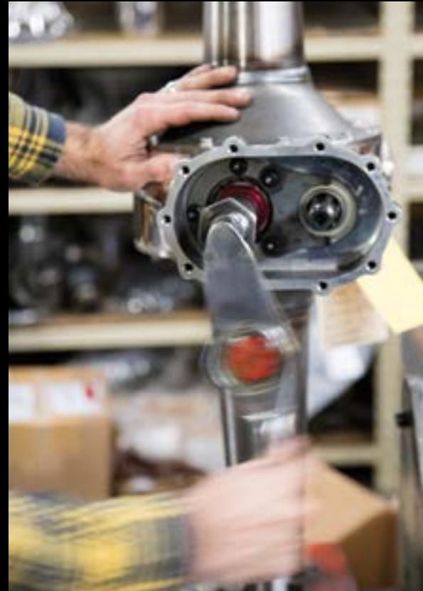
Each fastener is torqued to the proper specs and preloads to ensure correct alignment. Stainless steel ARP fasteners are available as an upgrade to Winters' standard hardware. Here longtime employee Andrew Staples attaches steel bells and torques the pinion nut on a V8 rear before the retainer and spur gears are installed.
