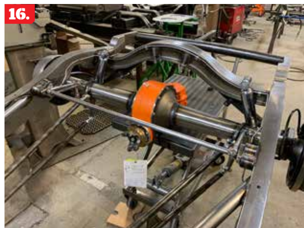
16. Tesar and Caraballo wrapped up the job with the installation of a Wide Track antiroll bar from Johnson's Hot Rod Shop.
