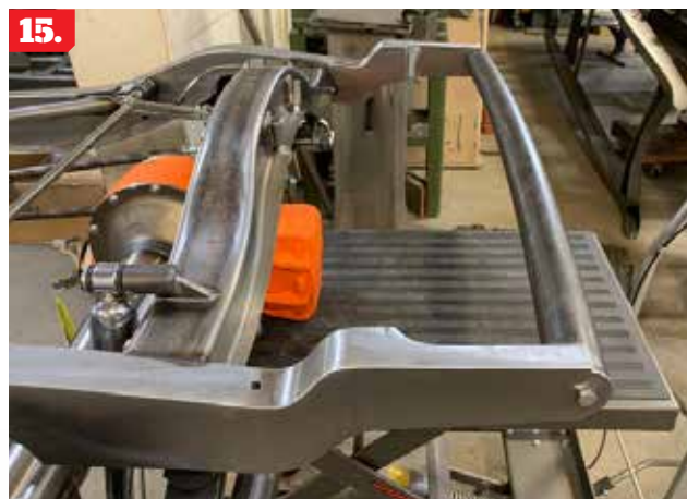
15. It makes little sense to invest in that much axle only to hide it with a tank (that needs modifying to accommodate the spur-gear housing). So, Tesar and Caraballo eliminated the tank, kicked up the framehorns to follow the trunk floor, and bobbed them to end at the apron. Precision slip-rolls these 2-1/8-inch spreader bars to follow the apron's curve.
